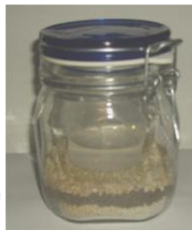
Schematic and real Biometer flask set up for simulated soil burial biodegradation tests.
